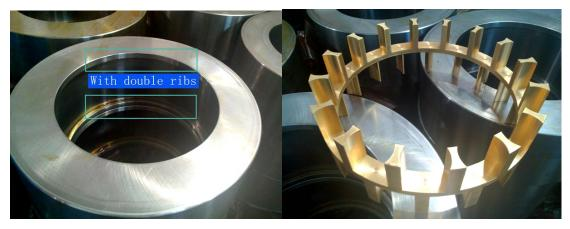
3. With special design of cage structure.
